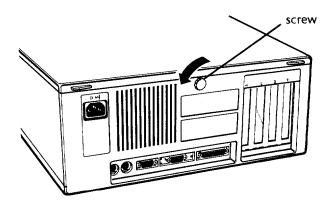
5. The cover is also secured by two latches on the back of the cover near the corners. Press both latches inward and then lift up the cover from the back panel. You might meet some resistance from the grounding tabs along the inside of the cover.
